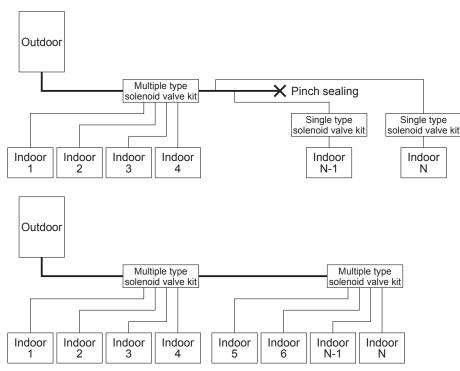
ex)Total allowable capacity=total capacity of indoor 1-indoor N
