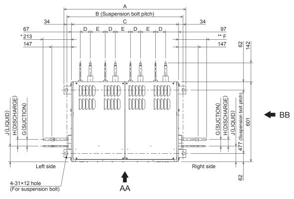
\* In case of right side connection. \*\* Including the protection tubes when connecting to the left side.
