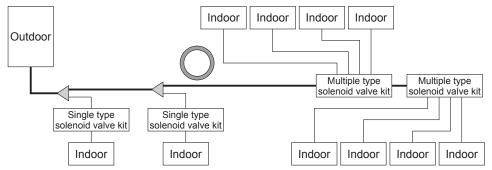
Multiple type solenoid valve kit before the distribution joint is disapproved
