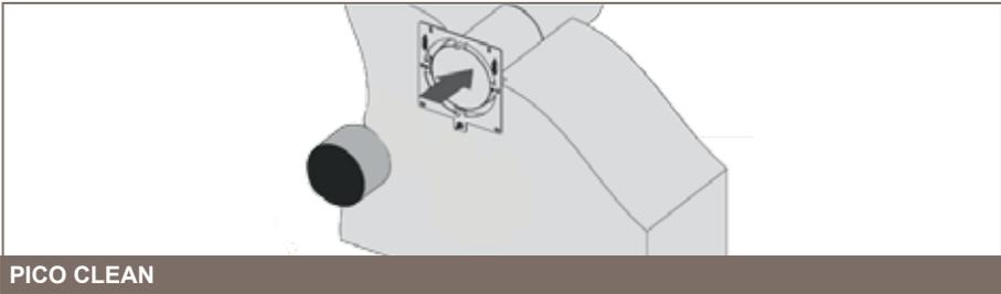
7) Attach the fan unit to the wall ring
