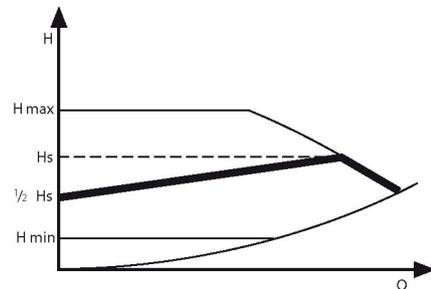
During start-up of the plant is recommended to put the speed selector to the maximum. The setting of maximum head is then performed with compressor capacity 100%, all distribution valves opened and the utilities turned on by checking the temperature difference between water send and return, that must be between 4 to 7 °C.
