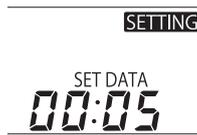
Within few minutes the prompt SETTING will appear and flash on the control panel of the external unit. This signal will cease within a maximum time of 4-5 minutes once the panel has correctly communicated with the external unit.
