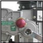
3. Also make sure that the emergency stop button is pulled towards you. In case you are not able to pull towards you the red emergency button with one hand, lightly press the trigger button of the joystick and with the other hand slightly turn the emergency button and pull. This maneuver does not cause any damage to the unit, but allows you to attach the gearbox.
