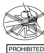
Conductor over insert
