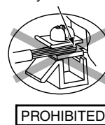
Conductor not fully insert
