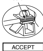
Conductor fully insert
