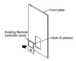
2. Press from front to fix the Remote controller cover 6 on the front plate.
