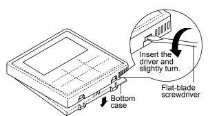
Remove the wiring between Remote controller and Indoor Unit terminal. Remove the bottom case from the Control board cover by loosening the screws. (3 pieces)
