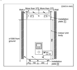
The centre of installation plate should be at more than 375 mm at right and left of the wall.
