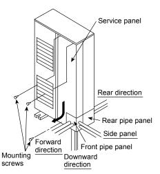
Close the tube joining area with putty heat insulator (local supply) without any gap as shown in right figure. (To prevent insects or small animal entering.)
