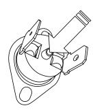
Use test pen to push this button for reset Overload protector (11).
