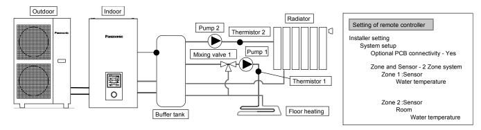
Connect floor heating or radiator to 2 circuits through buffer tank as shown in figure. Install pumps and thermistors (specified by Panasonic) on both circuits.
