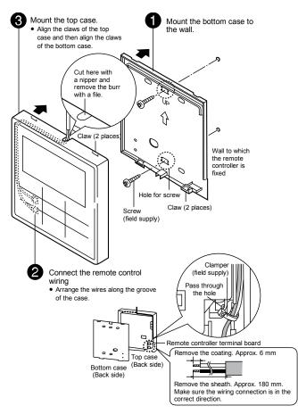
For embedded type **Preparation:** Make 2 holes for screws using a driver.
