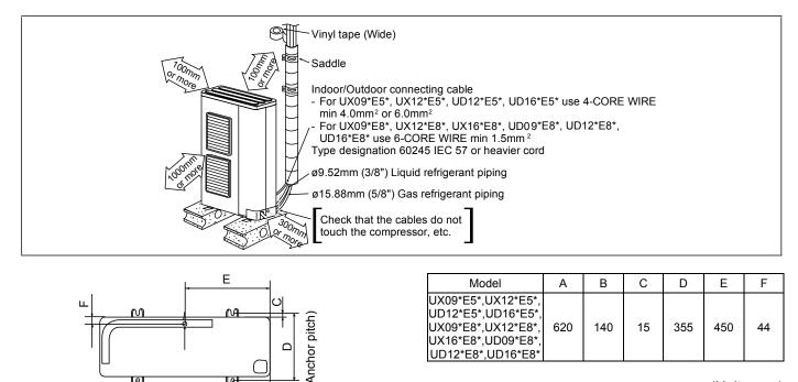
A (Anchor pitch) (Unit : mm)
