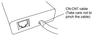
5. Use the included cord clamp to fix the CN-CNT cable to the wall.
