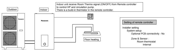
Connect floor heating or radiator directly to the indoor unit.
