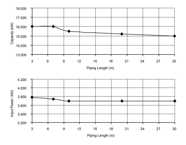
Cooling Characteristics at Different Piping Length Condition
